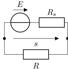
Pour  $R = 50\Omega = R_s$ , on a  $s = \frac{E}{2}$ . Pour  $R = 5,0\text{k}\Omega = 100R_s$ , on a  $s = \frac{100}{101}E = 0,99E \approx E$ .
